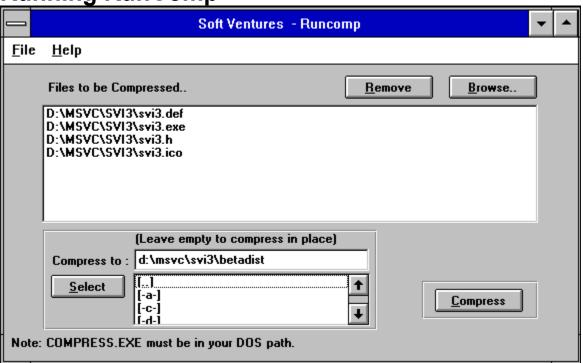
The object of the game here is to make a list of the file you wish to have compressed. Then click on 'Compress' and RunComp will batch up a COMPRESS.EXE run to do the work.
